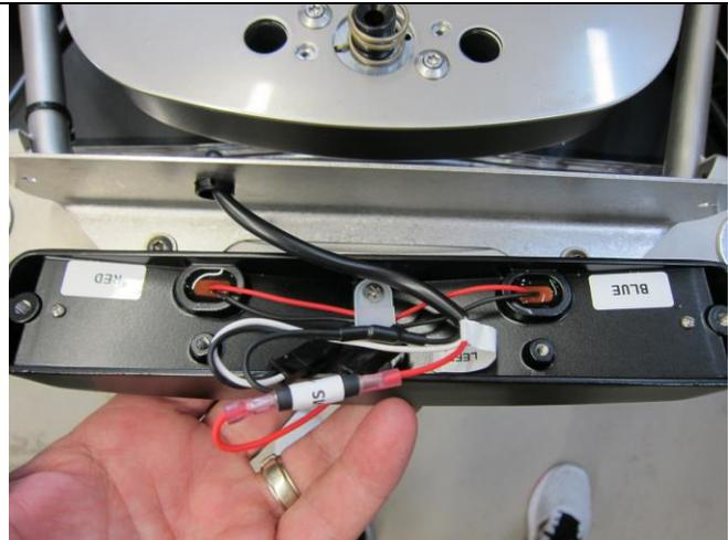
Because the two rear-facing emergency lights in the rear pod share the same output node as the duplex auxiliary light, a diode must be placed on any red emergency light wire before it plugs into the flasher board. Identify the red emergency light and the wire powering it – it connects to the center of the three plugs on each side. There is little room here, so cut the black wire as shown at right and strip back 1/2". Yes, on this light, the black wire is the + wire.
